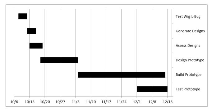
The Department of Dental Hygiene wants a working prototype by December 15. The first task of the design team is to test the Wig-L-Bug and analyze the power draw. After that, multiple designs will be evaluated. By October 17, a final design will be chosen and worked out. The team will begin building the power supply by November 4. Testing will start by December 1<sup>st</sup>. Two weeks will be sufficient time to complete the power supply.
